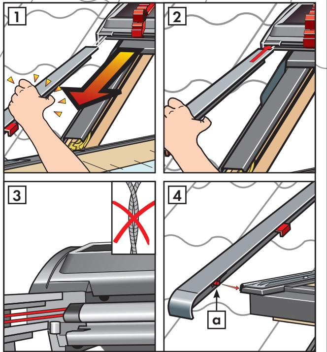
**English:** Pull side channel downwards (1). **It is necessary to pull the side channel hard.** Lift the awning top cover and slide the side channel straight into the groove in the top cover (2). Ensure that the cords do not cross each other and that they are positioned in the top cover (3). Snap sliding device (a) onto the bottom bracket (4).
