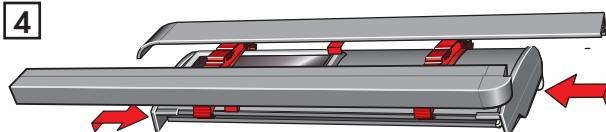
**English:** Remove end covers from both sides (1). Place adapter on axle and turn into position (2). Fix adapter with screw supplied (3). Refit end covers (4).
