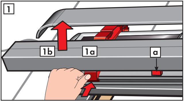
**English:** Disengage the right hand channel from the transit brackets (1), turn and hold parallel to right hand side frame (2). Do **not** remove the transit device (a) at this stage.
