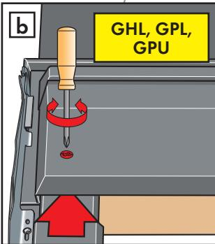
**English:** Loosen screws in top cover (a) or (b). Fit window covers using existing screws. Re-tighten top cover screws.
