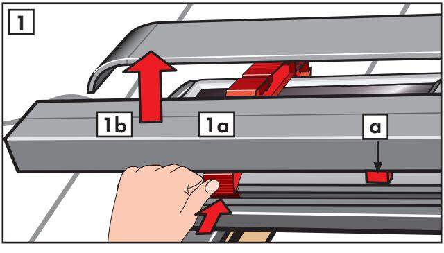
**English:** Disengage the right hand channel from the transit brackets (1), turn and hold parallel to right hand side frame (2). Do **not** remove the transit device (a) at this stage.
