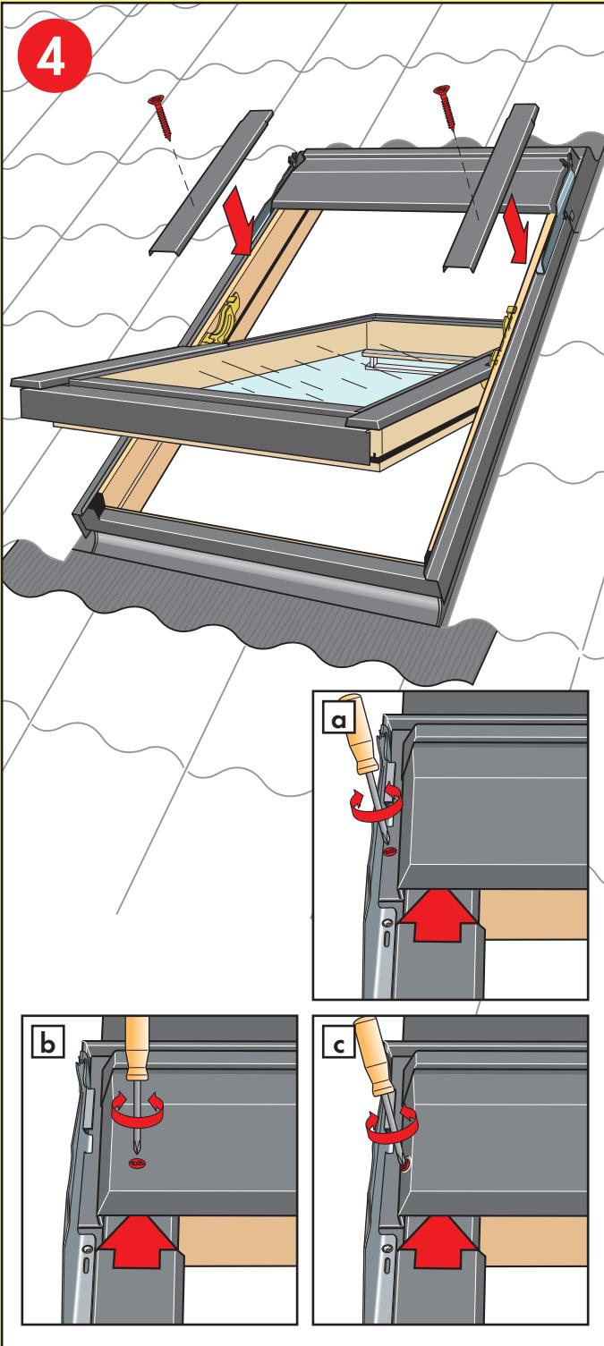
**English:** Loosen screws in top cover (a), (b) or (c). Fit window covers using existing screws. Re-tighten top cover screws.
