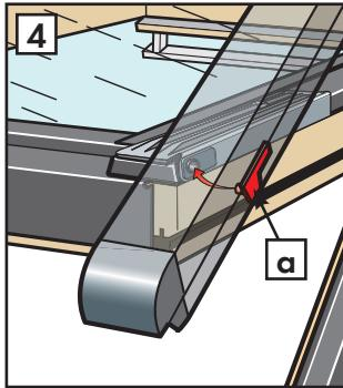
**English:** Pull side channel downwards (1). **It is necessary to pull the side channel hard.** Lift the awning top cover and slide the side channel straight into the groove in the top cover (2). Ensure that the cords do not cross each other and that they are positioned in the top cover (3). Snap sliding device (a) onto the bottom bracket (4).
