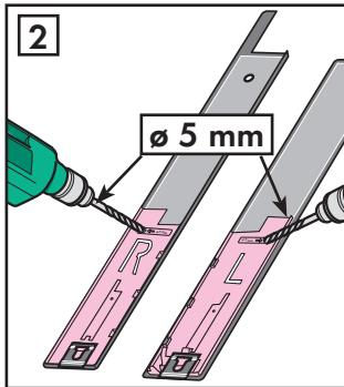
**English:** Fit distance sheets (**R** and **L**) on the underside of the covers. Slide the sheets completely down into the cover brackets (**1**). Drill holes, through the covers, at the marks using a Ø 5 mm drill (**2**).
