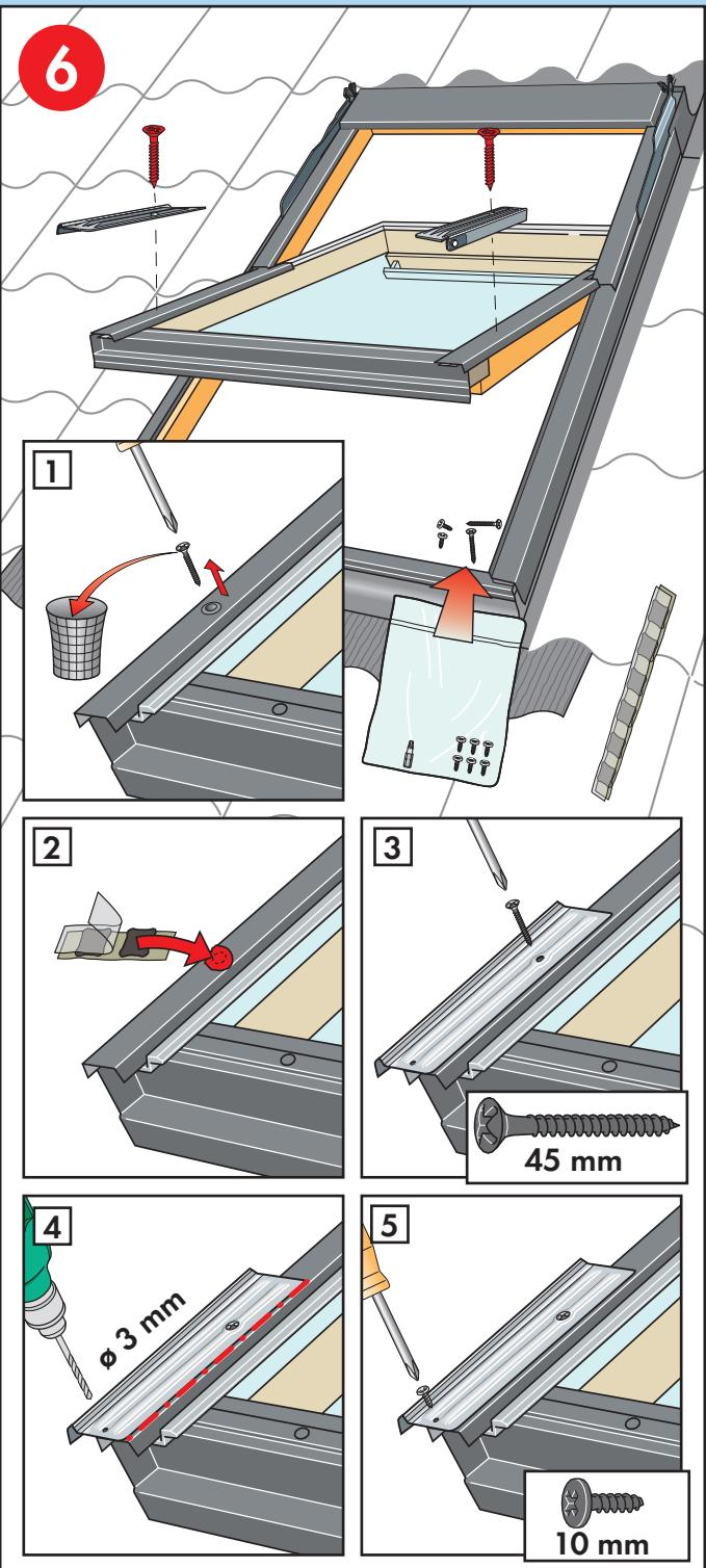
**English:** Remove and discard cover screws (1). Place sealant on screw holes (2). Fix bottom brackets with 45 mm screws supplied (3) and adjust so that they are parallel to the cover. Drill hole in cover through hole in bracket (4) and fix bracket with 10 mm screw supplied (5).
