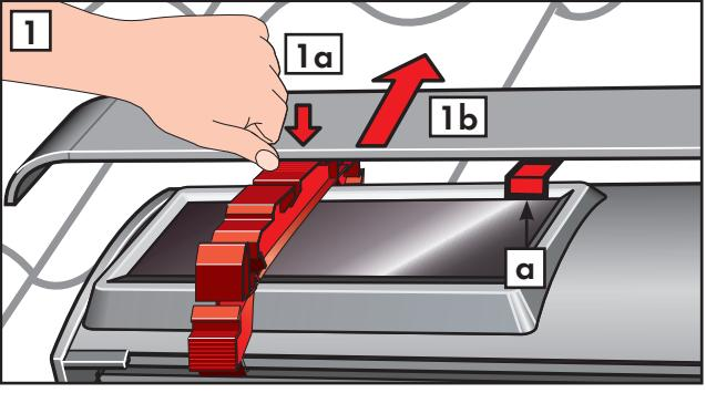
**English:** Disengage the left hand channel from the transit brackets (1), turn and hold parallel to left hand side frame (2). Do **not** remove the transit device (a) at this stage.
