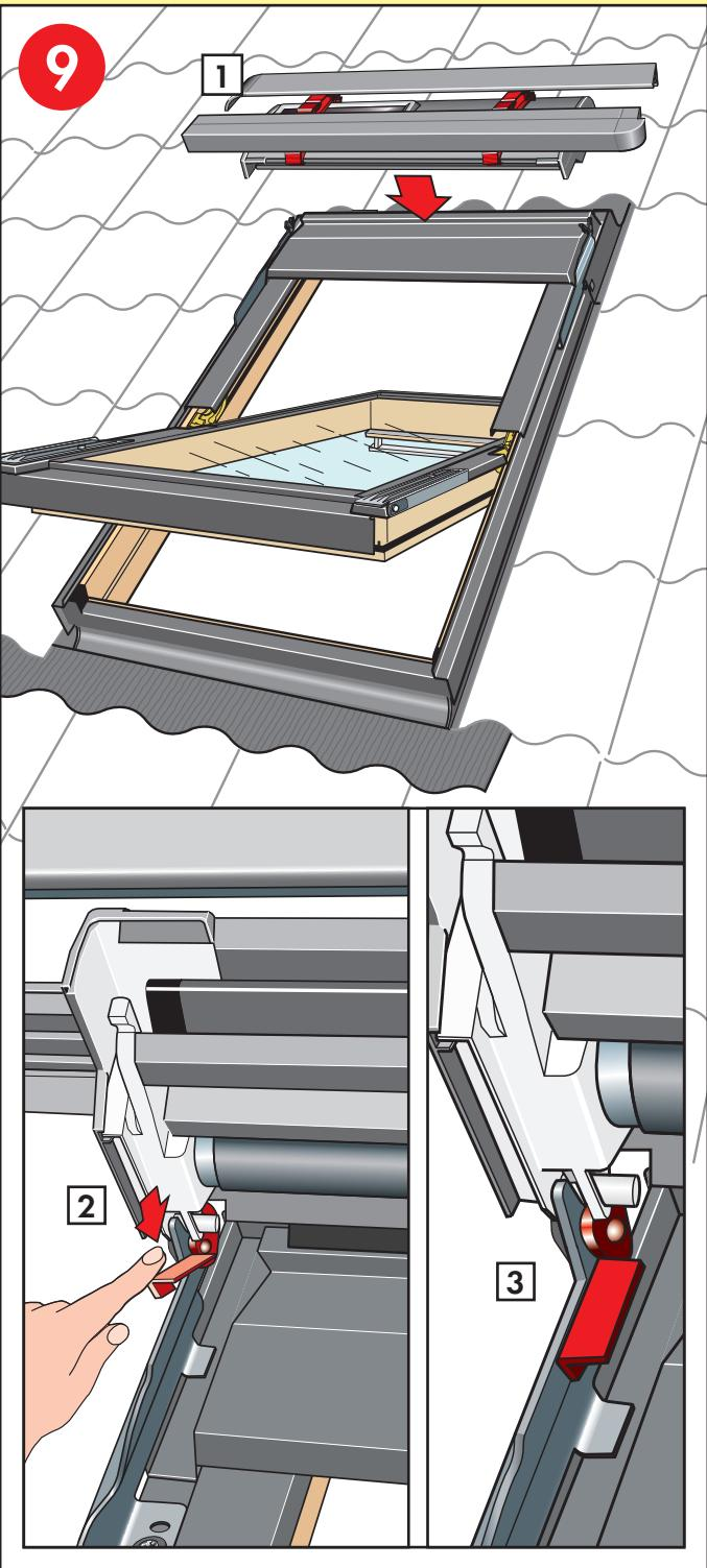
**English:** Position awning blind (1). Fit the awning blind into the bracket and lock it in place (2). Ensure that the locking bracket is pressed fully home (3).
