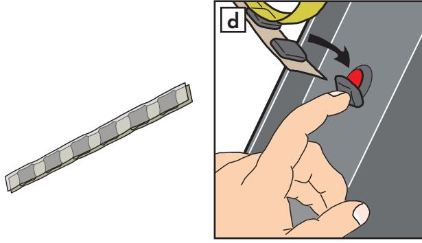
**English:** Remove covers indicated temporarily (**a**). Remove cover screws except the top cover screw (**b**). If there is a mark at the top instead of a screw, drill hole through mark (**c**). Place sealant on **all** screw holes (**d**).
