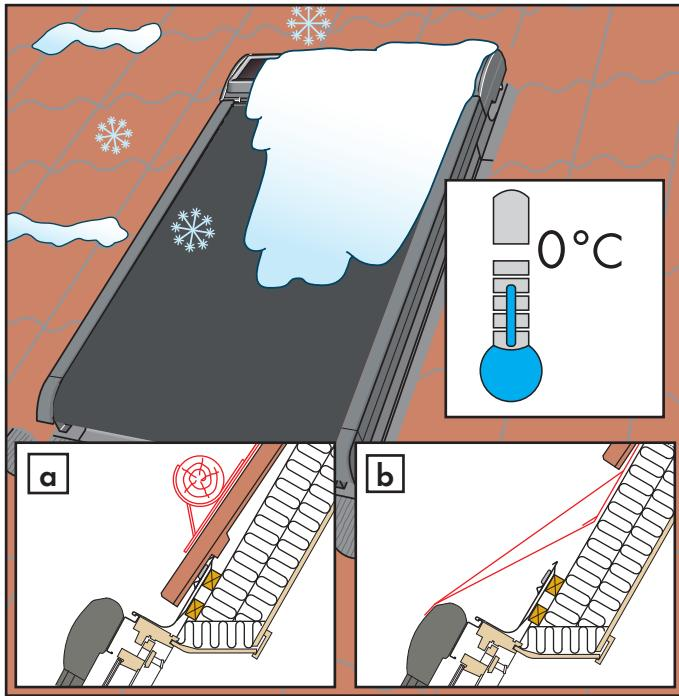
**ENGLISH:** As a precondition of avoiding any damage to the awning blind in very cold regions and in regions with heavy snowfall, either a snow stop or snow-wedge must be installed above the awning blind **a**, **b**. The awning blind is protected against overload, and will stop automatically if it is blocked.
