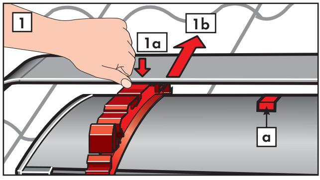
**English:** Disengage the left hand channel from the transit brackets (1), turn and hold parallel to left hand side frame (2). Do **not** remove the transit device (a) at this stage.
