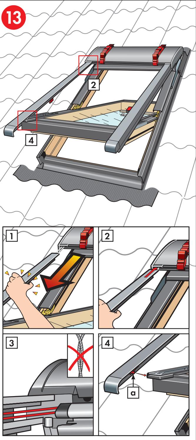
**English:** Pull side channel downwards (1). **It is necessary to pull the side channel hard.** Lift the awning top cover and slide the side channel straight into the groove in the top cover (2). Ensure that the cords do not cross each other and that they are positioned in the top cover (3). Snap sliding device (a) onto the bottom bracket (4).
