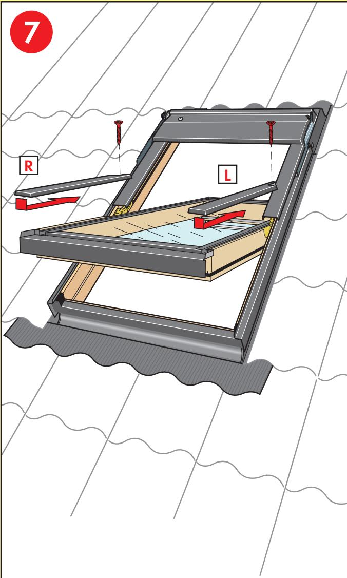
**English:** Refit the covers (1), then drill hole, in sash, through the covers using a Ø 3 mm drill (2).
