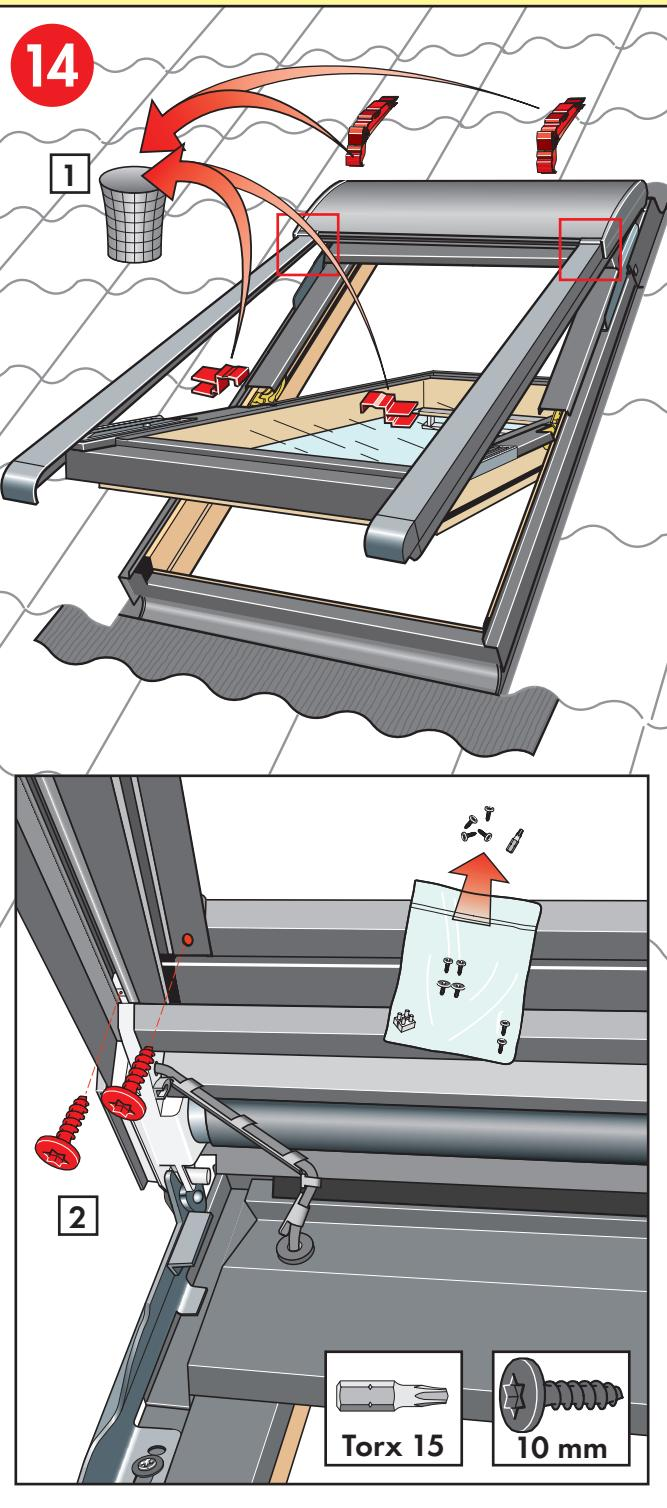
**English:** Remove and discard transit straps and devices (1). Fix side channels with screws supplied (2).
