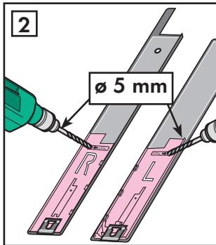
**English:** Fit distance sheets (**R** and **L**) on the underside of the covers. Slide the sheets completely down into the cover brackets (**1**). Drill holes, through the covers, at the marks using a  $\varnothing$  5 mm drill (**2**).
