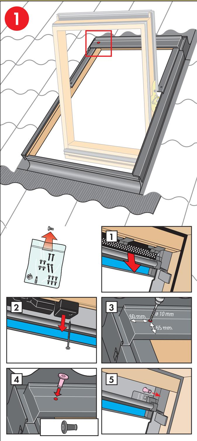
**English:** If the window has been fitted with a black screen profile, remove this temporarily (1). For GGL/GGU INTEGRA® windows, remove the connection box temporarily (2). Drill hole (3), and fit rubber grommet (4). Pull grommet through from the inside (5).
