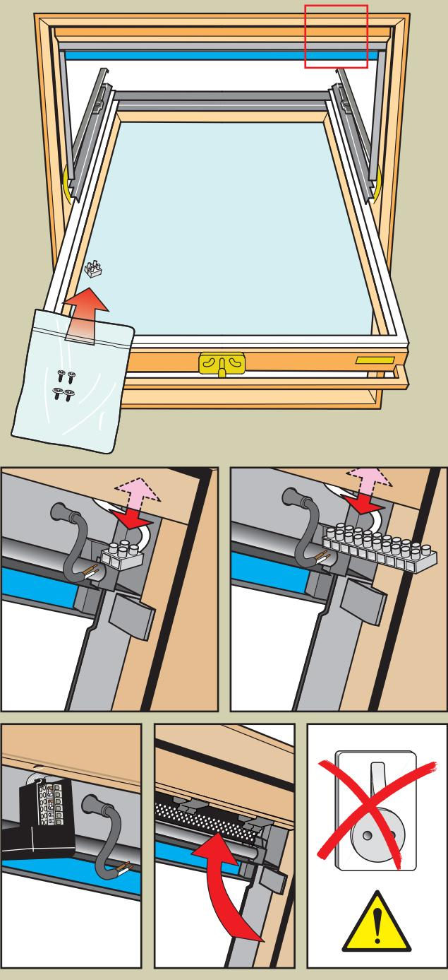
**English:** Connect the cable to terminal block or connection box. For connection to control system, refer to instructions for control system/remote control. If the window was fitted with a black screen profile and/or a connection box, refit profile/box.
