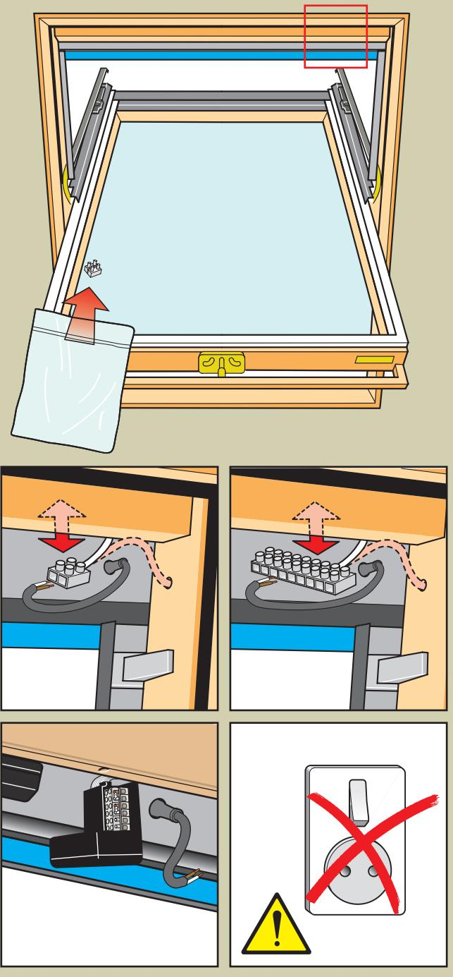
**English:** Connect the cable to terminal block or connection box. For connection to control system, refer to instructions for control system/remote control. If the window was fitted with a black screen profile and/or a connection box, refit profile/box.
