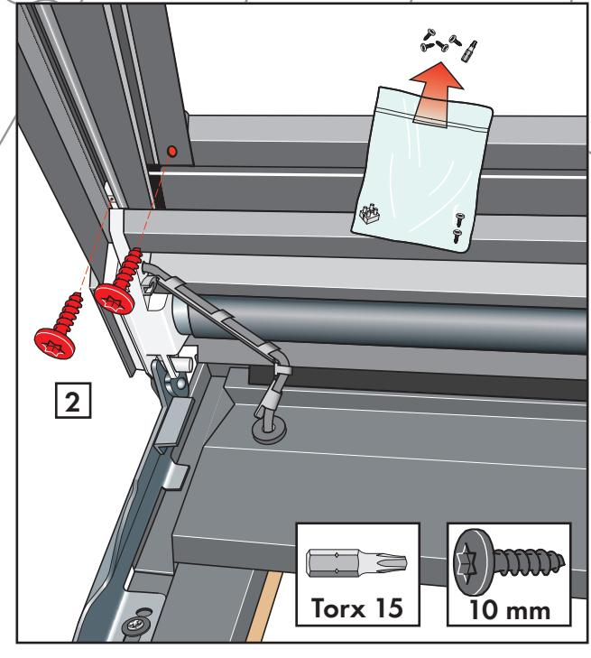
**English:** Remove and discard transit straps and devices (1). Fix side channels with screws supplied (2).
