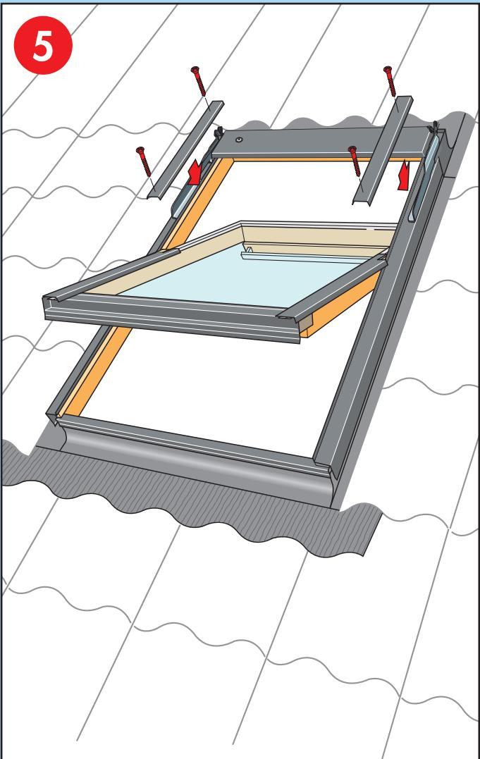
**English:** Loosen screws in top cover (a) or (b). Fit window covers using existing screws. Re-tighten top cover screws.
