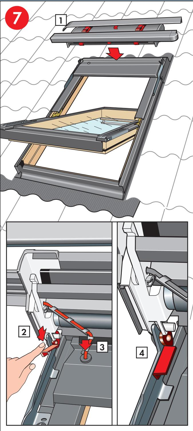
**English:** Position awning blind (1). Fit the awning blind into the bracket and lock it in place (2). Pull wire through grommet (3). Ensure that the locking bracket is pressed fully home (4).
