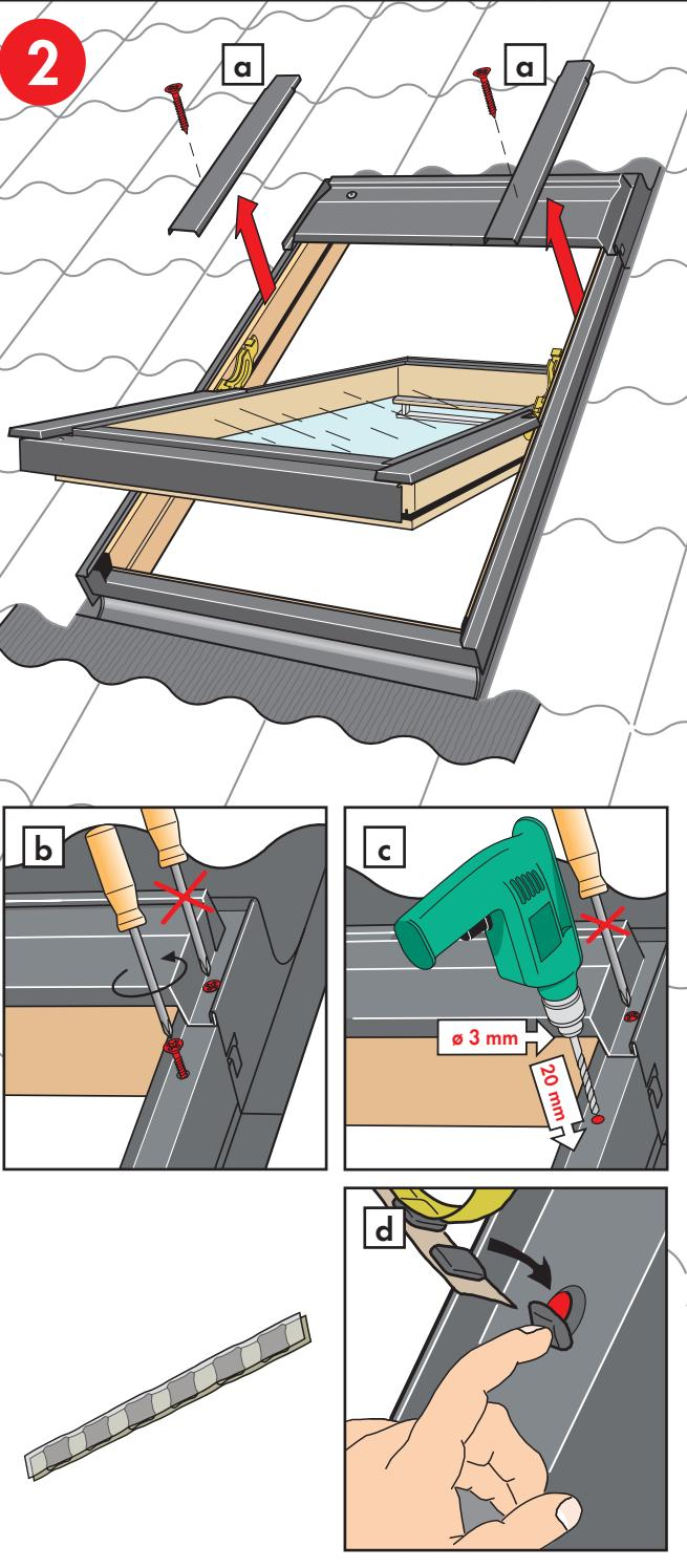
**English:** Remove covers indicated temporarily (**a**). Remove cover screws except the top cover screw (**b**). If there is a mark at the top instead of a screw, drill hole through mark (**c**). Place sealant on **all** screw holes (**d**).
