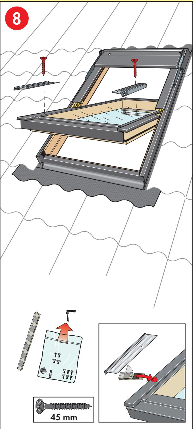
**English:** Place sealant on screw holes and fit bottom brackets with screws supplied.
