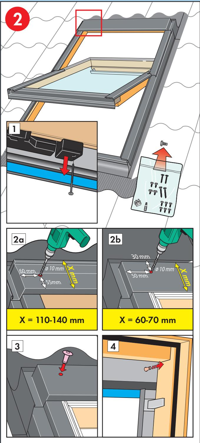
**English:** If the window has been fitted with a connection box, remove it temporarily (1). Position of hole depends on the width **X** of the top cover. Determine the width and drill hole (2a, 2b). Fit rubber grommet (3). Pull grommet through from the inside (4).
